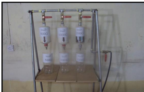
Figure 2: Magnetic water treatment device with three intensities.
