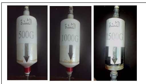
Figure 1: Magnetrons with three magnetic intensities of 500, 1000 and 1500 Gauss.
